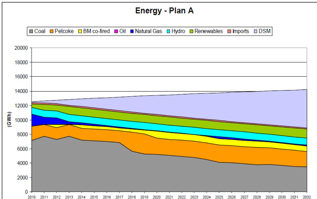
Figure 1: Sample DSM wedge from NSP's Integrated Resource Plan (NSPI 2009)
